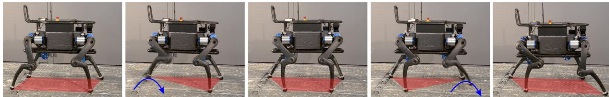
Figure 14. ANYmal can walk by moving one leg at the time and keeping the center of pressure within the support triangle.
