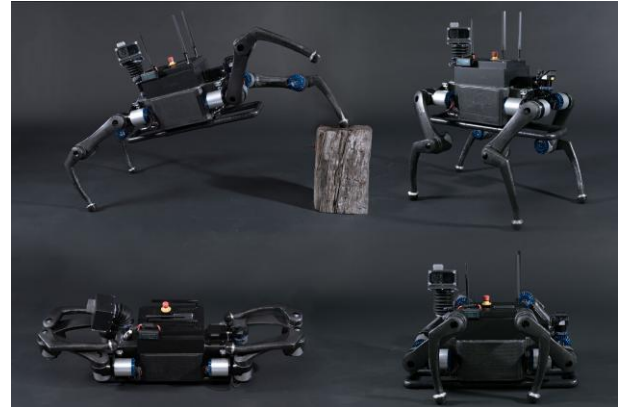
Figure 7. Full rotation in all joints of ANYmal allow for various configurations.
